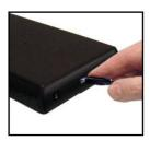
Plug the cable (USB or LAN) into the Freecom Network Drive XS.
